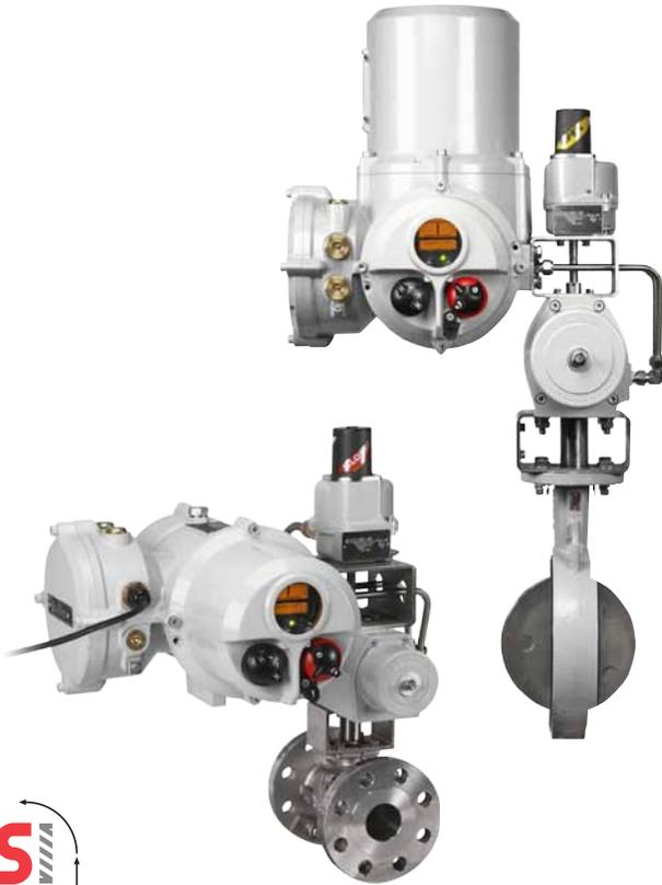
The SI-Q are compact and robust spring return actuators designed for all types of ball, butterfly, plug valves and dampers. Consisting of a self-contained electro hydraulic power module with a spring return scotch yoke drive the actuators are available as spring return clockwise, anti-clockwise or lock in last position. The SI actuators can also be configured for modulating control with a positioning resolution <0.2%.
