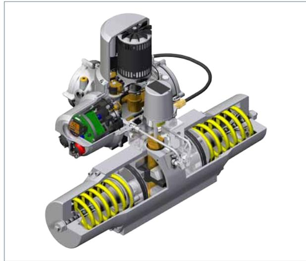
The actuators operate on a pump and bleed principle utilising a motorised vane pump to provide hydraulic pressure in one direction and spring-return in the opposite (bleed) direction.
